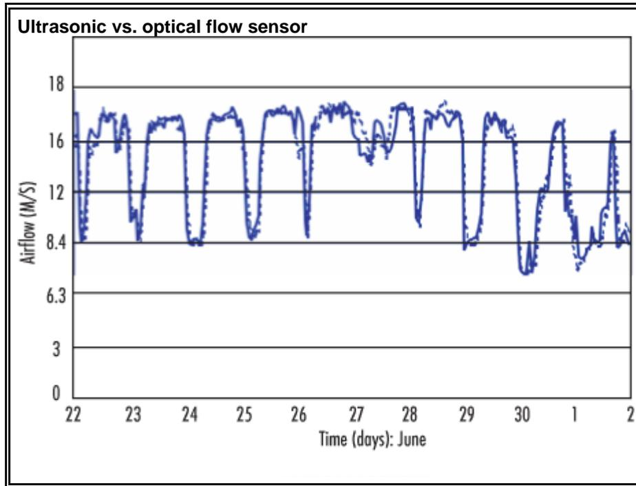
Ultrasonic technology measures the flow along the direction of the path and therefore requires some degree of angle. Therefore, the sensor is not measuring the true cross-stack velocity in a direct way. Pressure and temperature gradient also affect ultrasonic readings.
