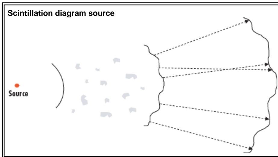
Photographs readily show the effect of scintillation or optical turbulence on a laser beam after traveling through the atmosphere. Instead of a uniform round disc, the beam is broken up and distorted by the turbulence. The strength of the atmospheric turbulence translates as a refractive index structure constant.
