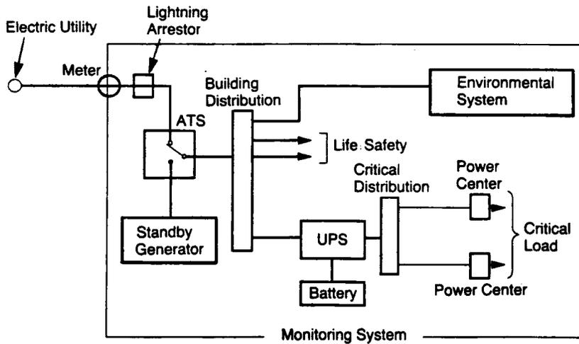
A typical IT Data Center is represented above in **Fig. 1**. We can see from the diagram that IT Data Centers are EMI/RFI-Surge protected environments. The IEEE Orange & Emerald Books recommend not only Lightning Arrestors, but also Delta-Wye transformer isolation on the UPS mains. The design of the Data Center's AC power distribution system protects the UPS from the effects of incoming EMI/RFI (electromagnetic & radio frequency interference) on the AC Mains and Bypass Input feeders.
